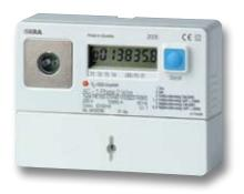
It is a single-phase multi-rate electronic active energy meter with an internal clock or two inputs for changeover of max. four tariffs. A seven-segment LCD and an optical interface are built-in.
