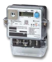
It is a single-phase multirate electronic meter of active energy and demand. It measures current and voltage. The internal clock enables changeover of max. four tariffs. A seven-segment LCD and an optical interface are provided.
