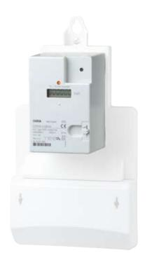
It is a three-phase single-rate electronic meter used for measurement of active energy. A simple plug-in connection complies with DIN VDE 0603-5. The meter can be connected to a single-phase or three-phase network. It is provided with a seven-segment LCD and a unidirectional optical interface.
