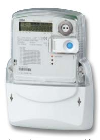
It is a three-phase multirate electronic meter used for measurement of active or active and reactive energy. A terminal block is available for a whole current or transformer connection. An internal clock is used for changeover of max. four tariffs. The meter is provided with a seven-segment VDEW display and an optical interface.
