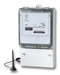
It is used for automatic reading of the ME/MT371 meter via  $3 \times 230/400 \, \text{V}$  low-voltage network. Readout data are stored in a non-volatile memory. On request, they are transferred to the AMM centre via a built-in GSM/GPRS modem or Ethernet interface. Up to 1024 meters can be connected to one concentrator. A built-in algorithm enables automatic recognition and installation of new meters, and automatic configuration of DLC network.
