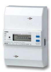
It is a single-phase multirate active energy electronic meter. Four tariff options are available in compliance with the Blue Tariff of Electricité de France (EDF). Instantaneous current and demand can be displayed. A ripple control receiver with 175 Hz carrier frequency and a communication interface for connection to the Euridis bus are built in. "Teleinformation" and 4 A relay outputs are provided.
