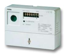
It is a single-phase single rate electronic active energy meter with a seven-digit mechanical register (6 + 1 decimal).
