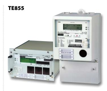
The electronic multifunction two- or three-element meter for CT or CT/VT connection is used for measurement of active and reactive energy and demand.
