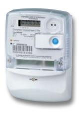
It is a single-phase multirate electronic active energy meter with four tariffs. A built-in ripple control receiver (216.66 Hz), a communication interface for connection to the Euridis bus and a 10 A relay output are provided.
