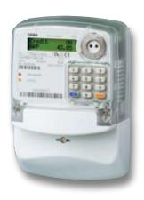
It is a single-phase multirate electronic prepayment active energy meter with an internal clock, four tariffs and one block tariff. A keyboard and an illuminated LCD are provided. A switching device (100 A) is built in. The meter is provided with an optical interface and a built-in GSM modem.
