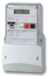
The electronic modular designed multifunction three-element meter is used for whole current, CT or CT/VT connection for measurement of active, reactive, apparent energy and demand as well as analysis of energy quality.
