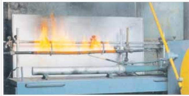
Testing of this property is conducted according to IEC 60331 which requires one meter of cable to be hanged and subjected to flame at 750 C for 90 min. and also according to BS 6387-which required one meter cable to be hanged and subjected to flame at  $950 \pm 40C$  for 180 min.
